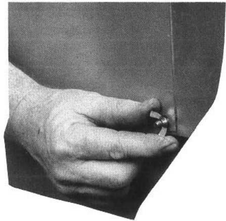
Figure 22: Securing Draft Hood to Canopy
