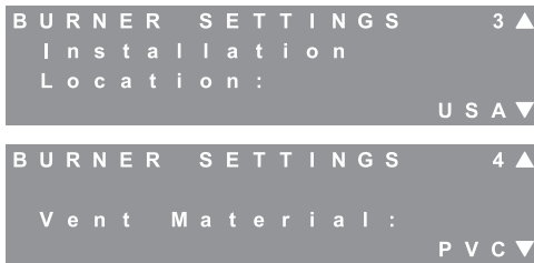
Figure 8.22: Burner Settings – Location & Vent Material
