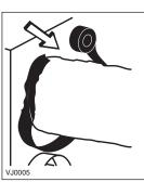
Apply duct tape to the joint making an airtight seal. Avoid compressing the insulation when pulling the tape tightly around the joint. Compressed insulation loses its R value and causes water dripping due to condensation on the exterior surface of the duct.
